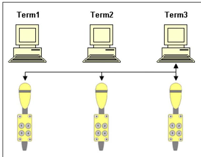
Figure 2 Multiple Dispensers Connected to a Single Terminal
