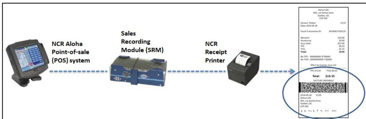
Figure 1 Sales Recording Module (SRM) Intercepting Transaction Example
