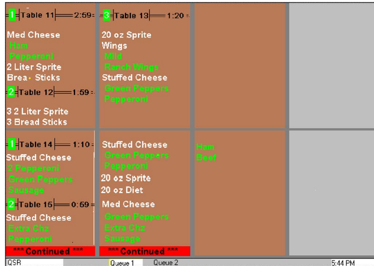
Figure 4 - 19 Top and Bottom Split Video Screen with Variable Cell Length
